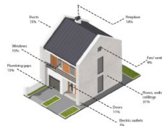
Figure 10: Air leakage in a house
